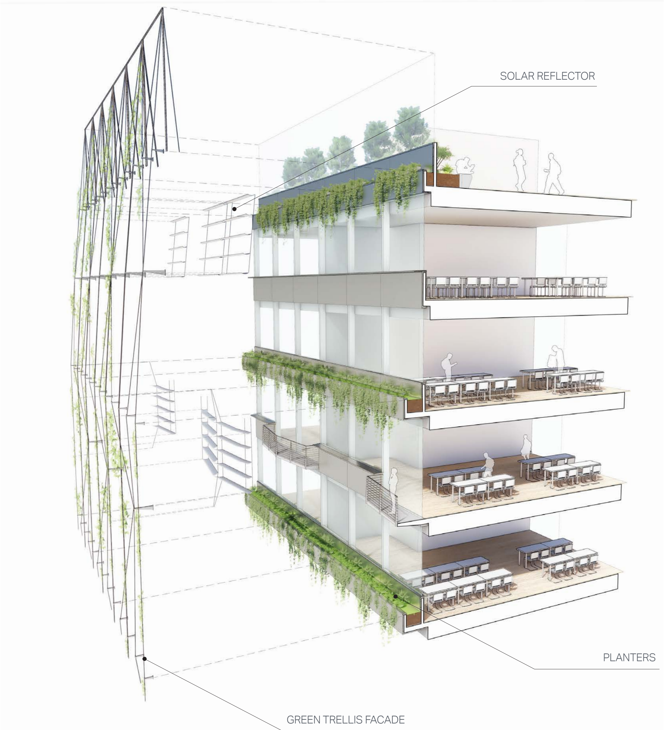
ACADEMIC TOWER: GREEN FACADE
